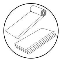
Unroll CCW EZRoof, cut into workable lengths and re-roll. Prepare roof deck for application by removing dust, dirt and all sharp protrusions. Deck should be free of oil and moisture.
