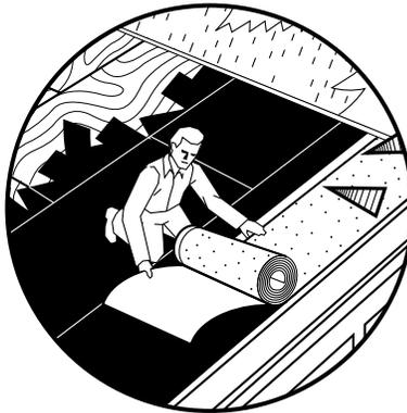
Position CCW EZRoof so that the end with the adhesive zip strip faces towards the overlap or top of roof.
